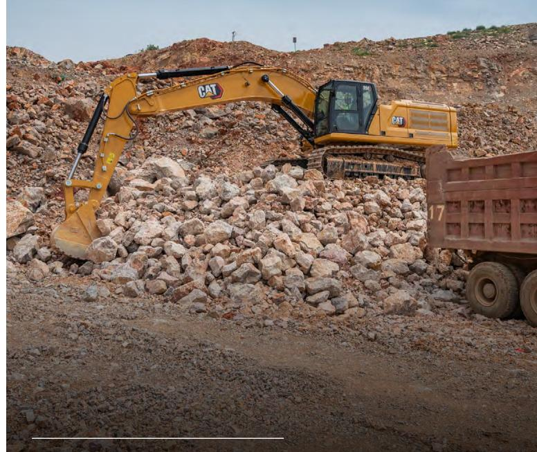
Engine Power (ISO 14396:2002) Operating Weight 309 kW (414 hp) 48 100 kg (106,000 lb)
